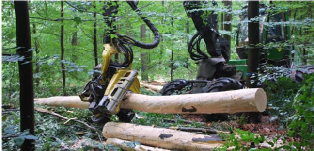
Abb. 1: Debarking Head Prototyp (H480C Aggregat John Deere)
